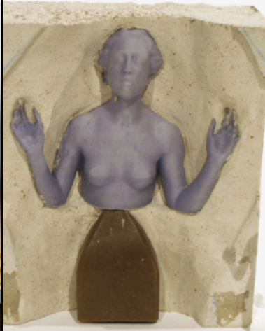
printed Torso (blue) embedded in molding material (grey), below one brown casting channel
