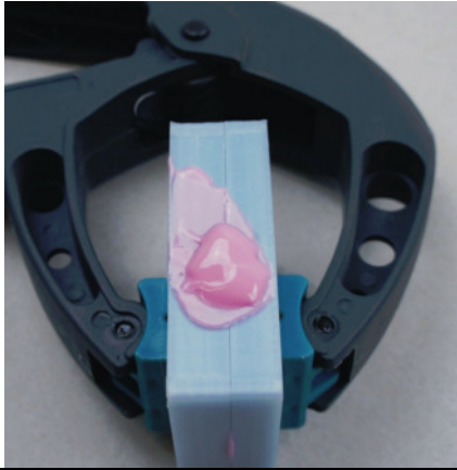
form printed from Moldlay (blue) filled with a 2K resin (pink)
