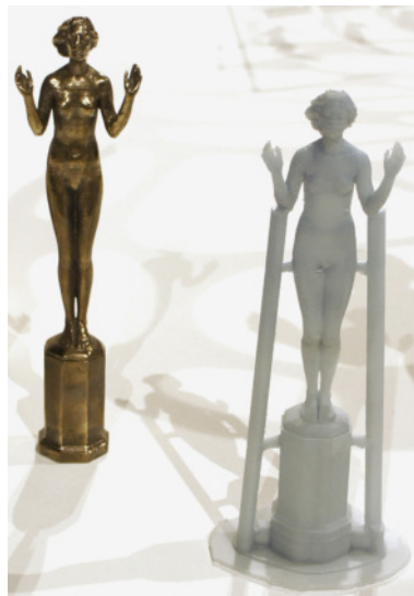
right: statue from Moldlay with casting channels left: ready casted and polished bronze statue
