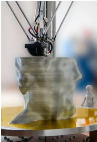
torso while being printed with a delta-printer
